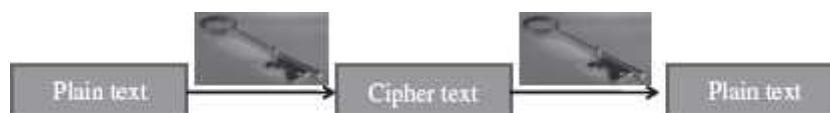
Figure 14.6 Secret key cryptography (uses a single key for both encryption and decryption)
