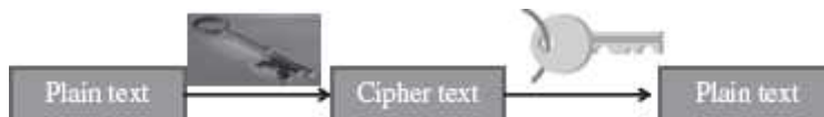
Figure 14.7 Public key cryptography (uses two keys—one for encryption and other for decryption)
