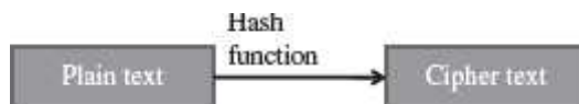
Figure 14.8 Hash function (have no key since plain text is not recoverable from cipher text)
