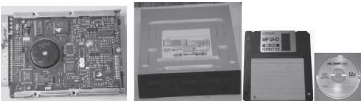
Figure 2.20 Storage devices (i) Hard disk drive, (ii) DVD drive, (iii) Floppy disk, (iv) CD
