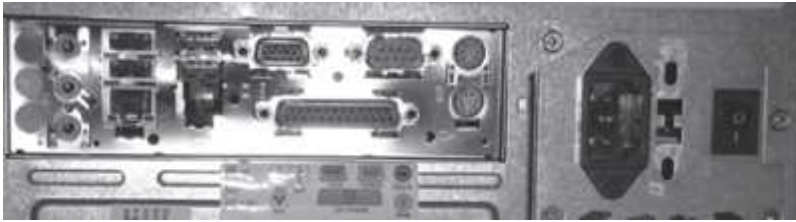
Figure 2.16 Ports on the rear side of a PC
