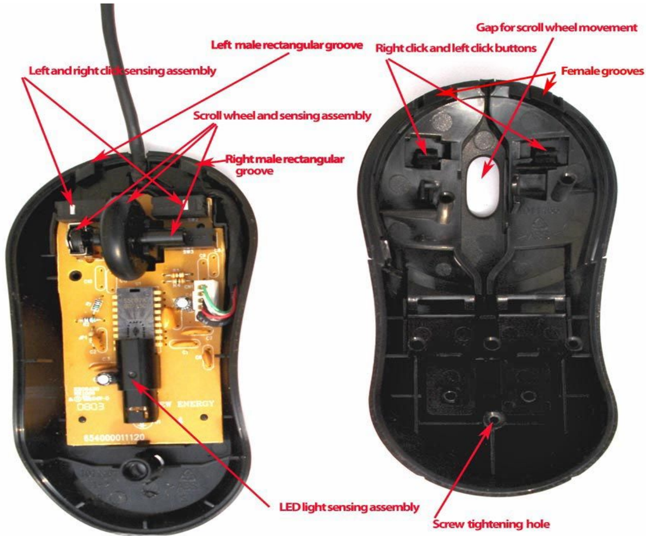
DELL Vostro 400 optical wired mouse internal view - top and bottom covers
